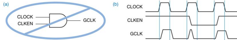
Bad clock gating: (a) simple-minded circuit; (b) timing diagram.
