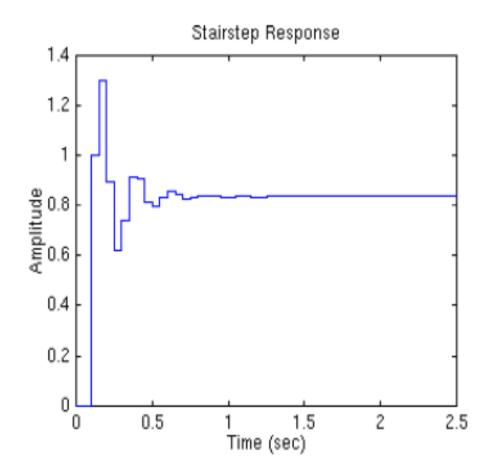
As you can see from the plot, all of the rise time, the settling time and the overshoot came out to be what we expected. We proved you here that we can use the locations of poles and the above three equations to analyze the transient response of the system.
