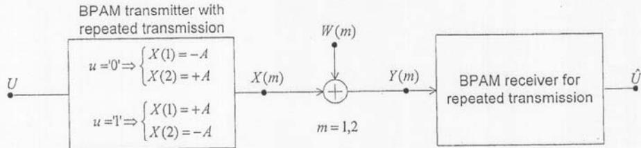
The signals  $X(1), X(2)$  at the transmitter output depend on the input bit  $U$  as follows:
