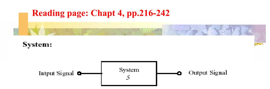
We look at a system as a black box which generates an output signal depending on the input signal and possibly some initial conditions.
