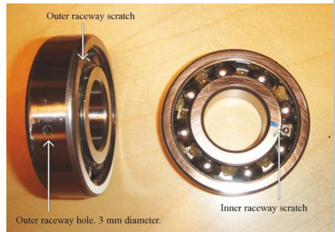
Fig.2 Outer raceway hole and inner raceway scratch
