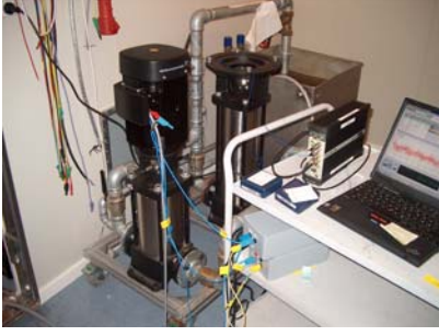
Fig. 3. The induction motor in a circulation system
