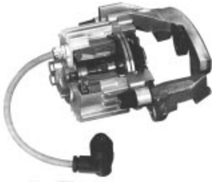
Fig. 15. Prototype of an electromechanically actuated wheel brake by Continental Teves
